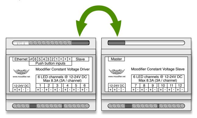
You can connect 2 types of slave units to the Moodifier Constant Voltage Driver, a Moodifier Constant Current Slave unit or a Moodifier Constant Voltage Slave unit. This adds great flexibility when designing your lighting since it enables a wide range of options for both constant current and constant voltage based LED lighting.
