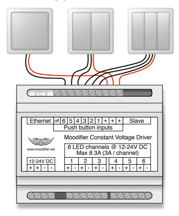
Moodifier Constant Voltage Driver with 6 connected push buttons that each activates/de-activates its own light scene.
