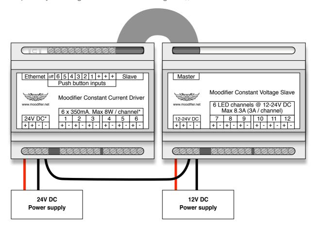
Interconnected Master and Slave units running different voltages and power supplies with common grounding.
