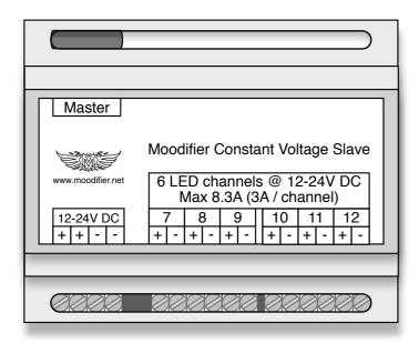
The DIN-rail mounted Moodifier Constant Voltage Slave seen from above with connectors facing up/down.
