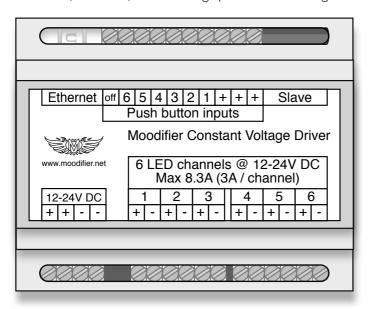
The DIN-rail mounted Moodifier Constant Voltage Driver seen from above with connectors facing up/down.
